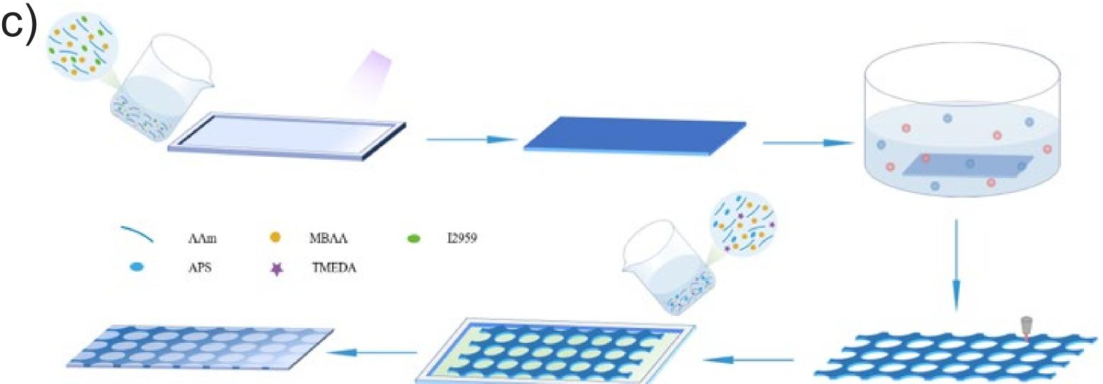
(c) Schematic illustration of the preparation process of the conductive composite hydrogel.
